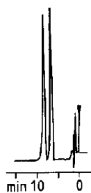
Fig. 9. Separation of the enantiomers of atenolol. Column, CHIRAL-AGP (100 \times 4 mm I.D.); mobile phase, phosphate buffer (pH 7.2) (0.01 M phosphate).
